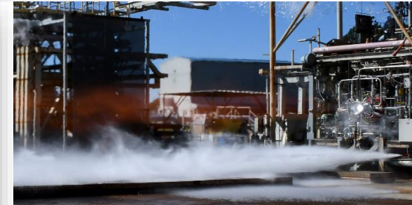
First successful Lox/Hydrogen hot fire test of a regen-cooled GRCop-84 3D printed MCC with an integral Electron Beam Free Form Fabrication (EBF3) deposited nickel superalloy jacket.
