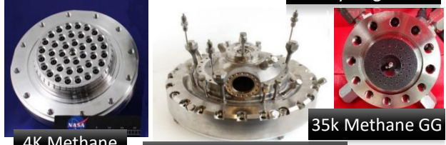
100 lb LOX Propane 1.2K LOX Hydrogen 20K AMDE Lox Hydrogen 4K Methane 20K AMDE Lox Hydrogen 35k Methane GG Injector Development
