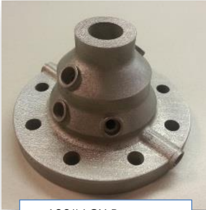
100# LOX Propane Injector Built 2012 Tested Nov 2013
