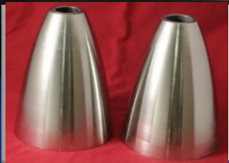
Freeform AM Deposition with Integral Channels
