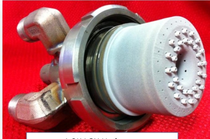
1.2K LOX Hydrogen First Tested June 2013 >7000 sec hotfire
