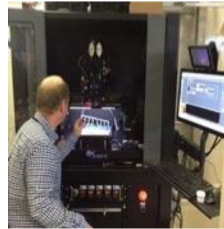
MSFC nScript multimaterial printer (4 heads and pick and place capability)
