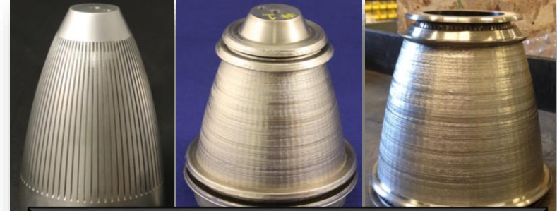
Additive Wire-based Channel Closeout
