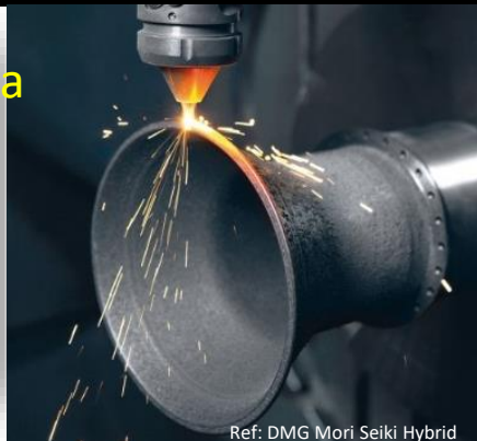
Large Scale Deposition: Blown Powder and Arc Deposition
