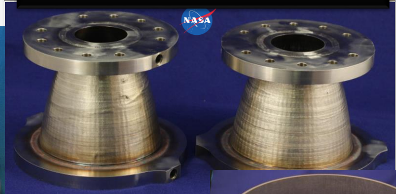
Additive Wire-based Channel Closeout
