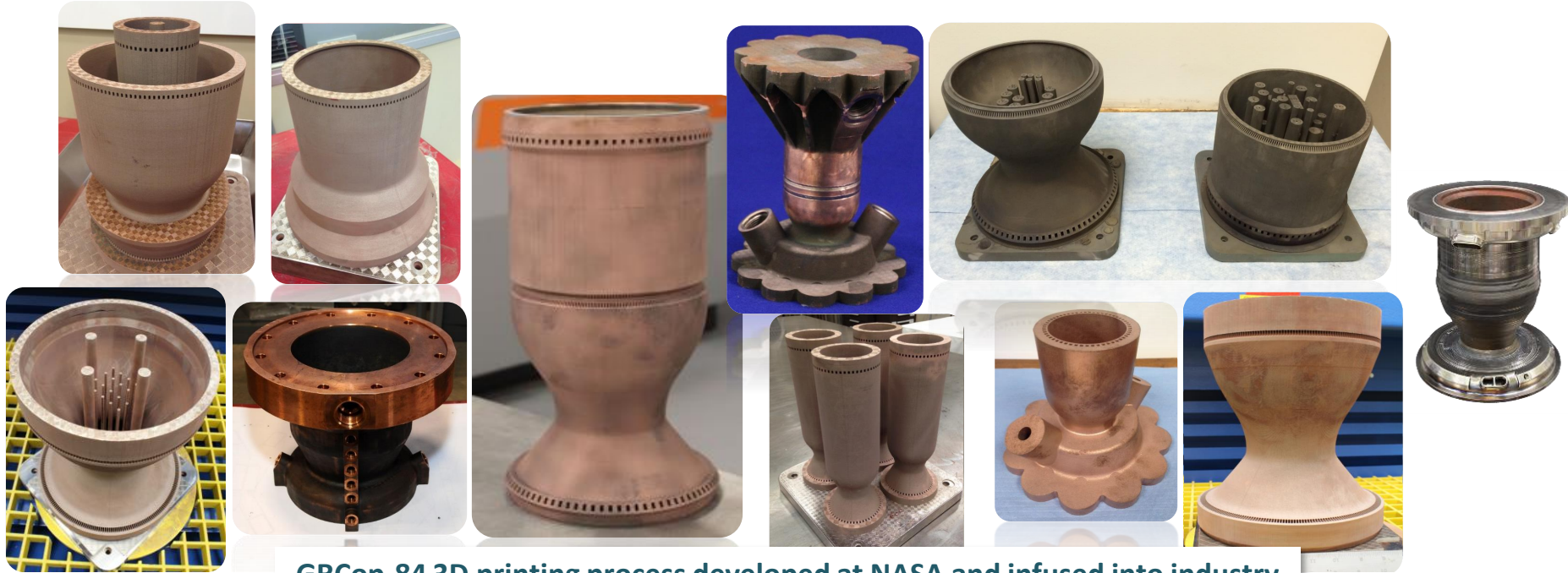
GRCop-84 3D printing process developed at NASA and infused into industry
