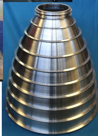
Freeform AM Deposition with Integral Channels
