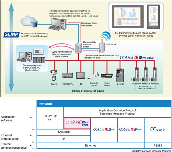
Cyclic communication on CC-Link IE Field network is realized by software. OThe system can be developed quickly, and a wide lineup of applicable devices can be developed easily. The communication can be done simultaneously with standard Ethernet TCP/IP communication (HTTP, FTP, etc.). OWiring for control is not required, and the Ethernet network can be unified.
