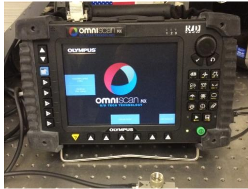
Olympus Omniscan Phased Array UT NDE
