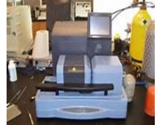
TA Q600 TGA/DSC with SPI 200amu mass spec
