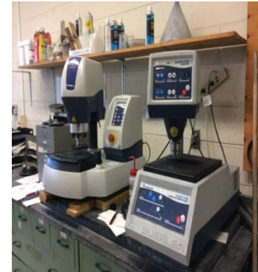
Sample preparation from Buehler Ecomet Auto Polishers (left); SPI Plasma Etcher (right)
