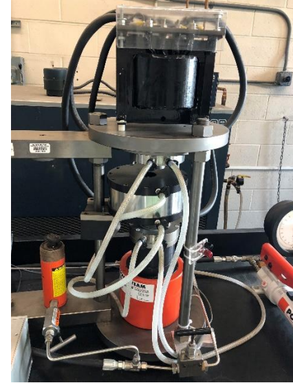
Depth of the Earth 3GPa 1800C Pressure Furnace
