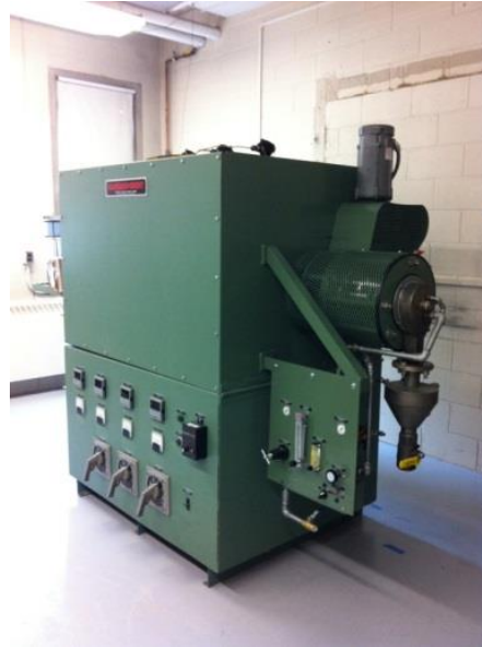
Unique Pereny Atmosphere controlled rotary calciner – 1000C
