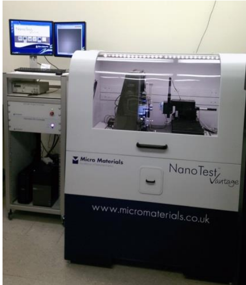
Micro Materials Vantage Nano/Microindentation System and Nano- impact System
