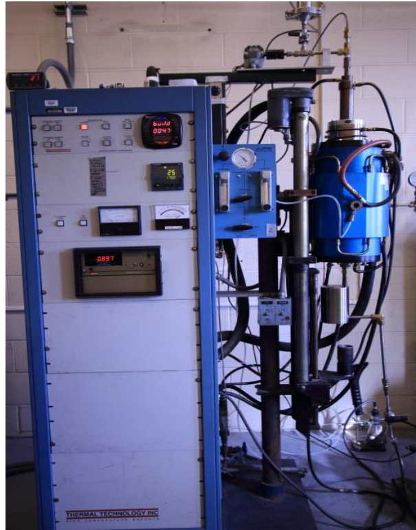
Small RCR Reactor (left) 10gram/2000C
