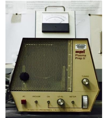
Sample preparation from Buehler Ecomet Auto Polishers (left); SPI Plasma Etcher (right)
