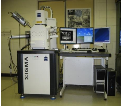
Zeiss Sigma FESEM with Oxford X-Max EDS and Oxford Nordlys EBSD
