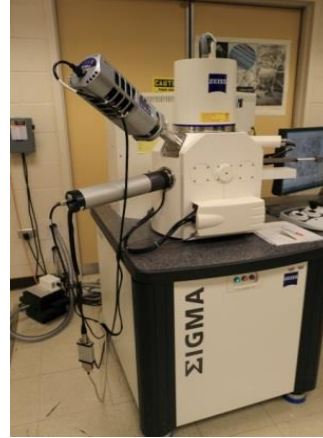
Zeiss Sigma FESEM with Oxford X-Max EDS and Oxford Nordlys EBSD
