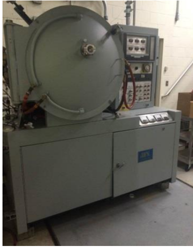
AVS Vacuum Furnace – 2000C
