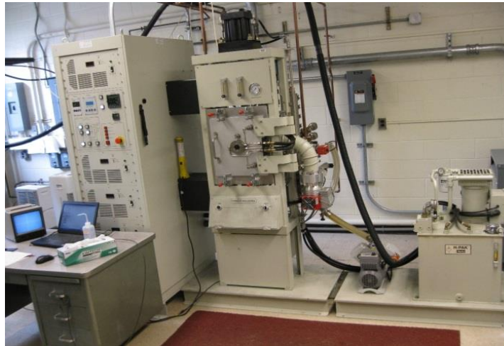
Thermal Technologies 10T Spark Plasma Sintering
