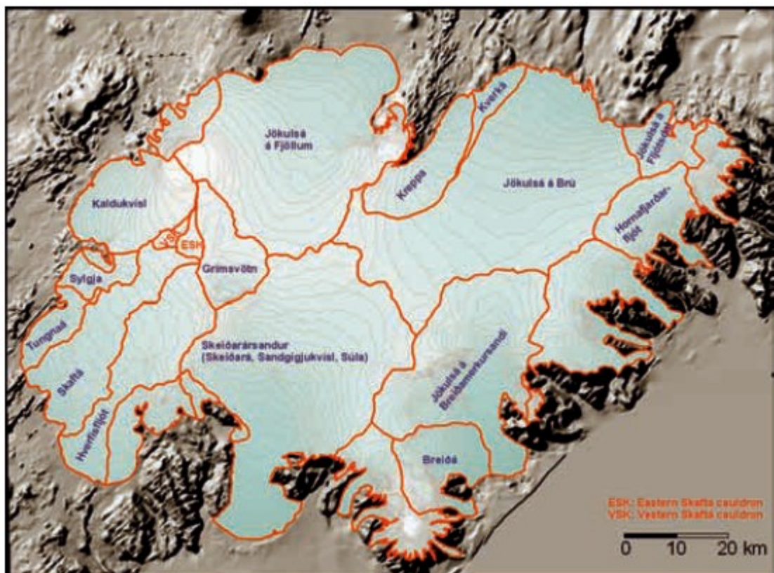
Figure 6: Water drainage basins at the glacier bed for the principal rivers draining Vatnajökull. Sub glacial water-filled cupolas, located under depressions in the glacier surface, collect melt water and periodically drain by means of jökulhlaups
