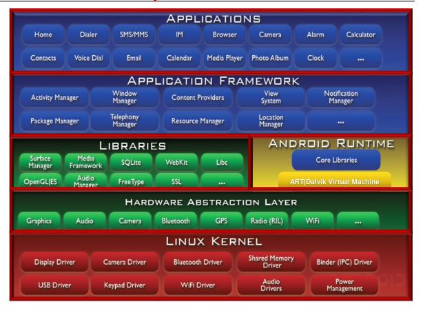
Android's architecture is structured in accordance to multiple layers
