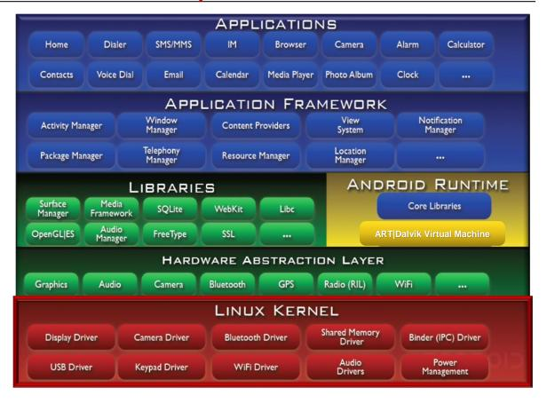
The Android Linux kernel controls hardware & manages system resources
