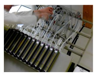
This test method is widely used for specification purposes like in ISO 8068, DIN 51515 part 1 L-TD, Siemens TLV 901304, Mitsubishi MS4 – MA – CL 001 002 003, General Electric GEK 107395A,... and is considered useful in estimating the oxidation stability of lubricants. Uninhibited oils will usually fail within 200 h, while high quality oils can exceed 5000 h – 10.000 h. However, it should be recognized that the correlation between this
