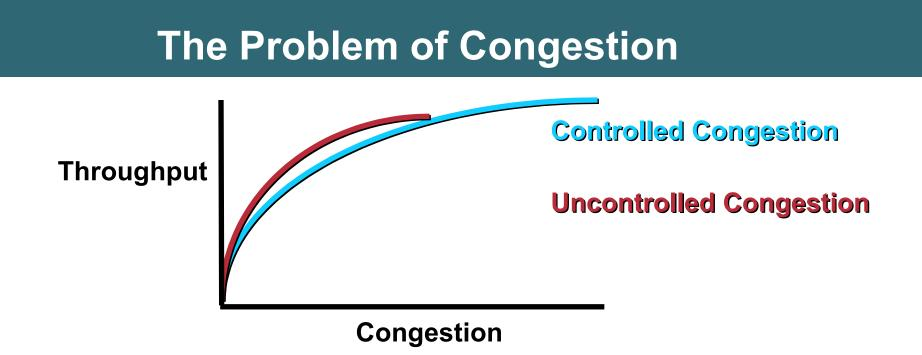
Uncontrolled, congestion will seriously degrade performance The system buffers fill up Packets are dropped, resulting in retransmissions This causes more packet loss and increased latency The problem builds on itself
