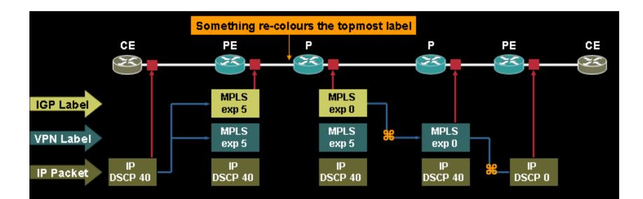
In both the MPLS-to-MPLS and the MPLS-to-IP cases, the PHB of the topmost popped label is copied into the new top label or the IP DSCP if no label remains.
