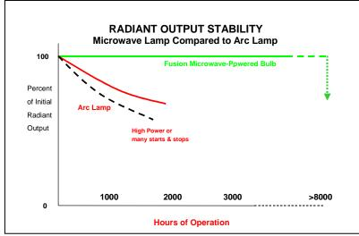
especially true for the longer wavelength, additive bulbs where the electrodeless bulbs are guaranteed for typically six to ten times the life of an arc type bulb and a UV LED system operates 20,000 plus hours.
