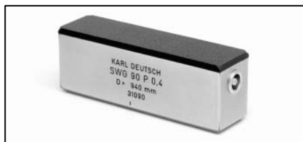
Surface wave probe for testing of railway wheels
