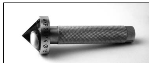
Cone probe for testing of railway wheels
