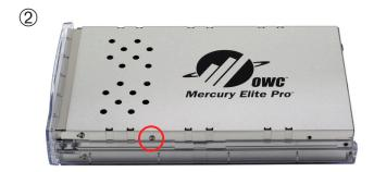
Then, remove the single Phillips screw securing the top metal shield. Lift up on it to remove, exposing the inside of the enclosure.
