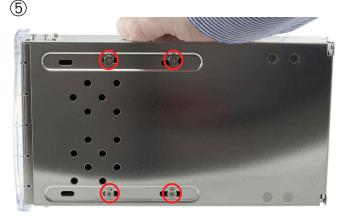
Turn the enclosure on it's side, removing the bottom plastic outer shell, and securing the drive you just placed into the enclosure with your fingers as shown above. Lift up on the hard drive mechanism and line the screwholes up with the cutouts on the bottom of the enclosure.
