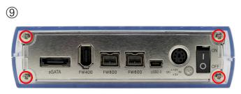
Insert the 4 screws through the top and bottom covers into the body of the OWC Mercury Elite Pro.
