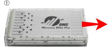
Remove the top cover from your OWC Mercury Elite Pro enclosure by sliding the top cover towards the rear of the unit.
