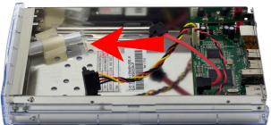
Remove the taped down packet of screws.
