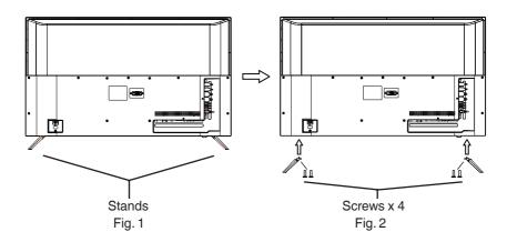
Be sure to follow the above instructions. Insufficient tightening or incorrect installation of the stand will not support your TV correctly, and could result in damage or injury from tipover.
