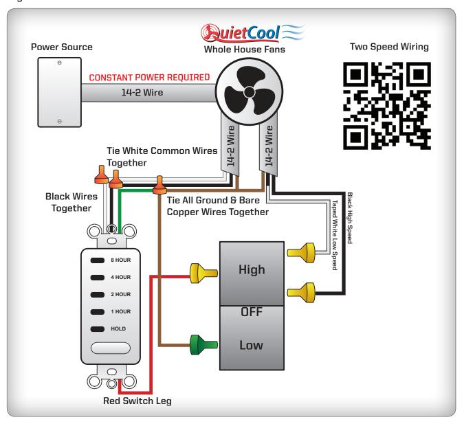
**6.** Attach the red leg wire from the timer to the top gold screw on the left of the switch. Finish up the installation of the timer and switch and switch cover plate.
