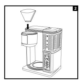
Place a #4 paper cone filter in the filter holder.
