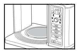
The Intelligent Warming Plate will automatically turn on during a Half or Full Carafe size of Classic or Rich brew. The Intelligent Warming Plate will adjust the heat it produces to avoid burning the coffee over time.
