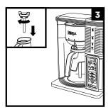
Twist the **Brew-Through Lid** clockwise onto the **Carafe** to lock into place and center the carafe below the brew basket.
