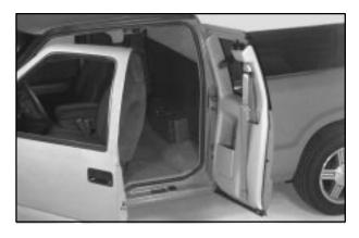
Your vehicle may be equipped with a side access panel for convenience in loading and unloading cargo.
