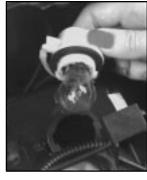
Twist the bulb socket counterclockwise to remove it from the headlamp assembly.
