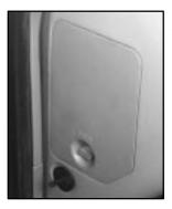
The instrument panel fuse block is at the driver's end of the instrument panel.
