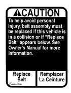
If you ever see a label on the driver's safety belt that says to replace the belt, be sure to do so. Then the new belt will be there to help protect you in a collision. You would see this label on the belt near the door opening.
