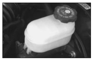
Your brake master cylinder reservoir is filled with DOT-3 brake fluid.
