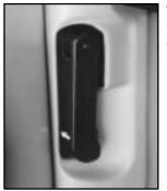
To open the hood, first pull the handle inside the vehicle on the lower left side of the instrument panel.
