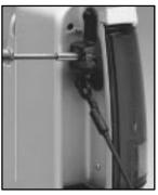
2. Remove the screws from the lamp assembly near the tailgate latch.
