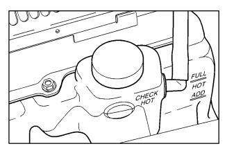
When the engine is cold, the coolant level should be at least up to the ADD mark. If it isn't, you may have a leak in the radiator hoses, heater hoses, radiator, water pump or somewhere else in the cooling system.
