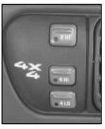
If your four-wheel-drive vehicle has the electronic transfer case, the transfer case switches are located to the right of the steering wheel.
