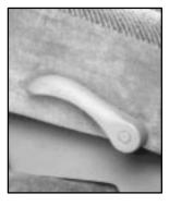
To adjust the front seatback, lift the lever on the outer side of the seat.
