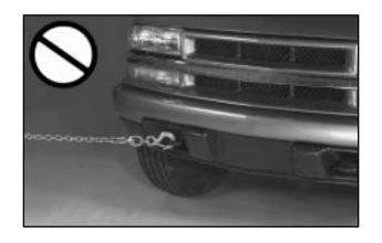
The recovery hooks, when used, are under a lot of force. Always pull the vehicle straight out. Never pull on the hooks at a sideways angle. The hooks could break off and you or others could be injured from the chain or cable snapping back.
