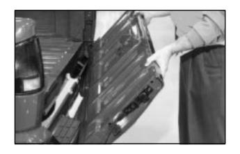
3. With the tailgate halfway down, pull the tailgate toward you at the left side and then move the tailgate to the left to release the right side.
