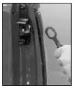
2. Remove both retaining cables. To remove each cable, turn it so the end faces the front. Then, push forward so the larger part of the hole is over the bolt. Pull the end over the bolt.
