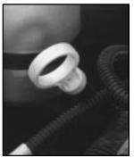
The oil dipstick on the "VORTEC" 4300 V6 engine is a yellow ring.
