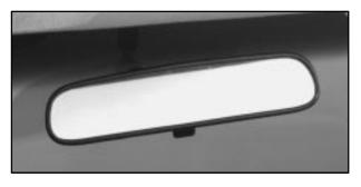
Pull the tab under the mirror toward you to reduce glare from headlamps behind you after dark. Push the tab away from you for normal daytime operation.
