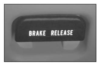
Pull the BRAKE RELEASE lever fully. It is located on the bottom of the driver's side of the instrument panel.
