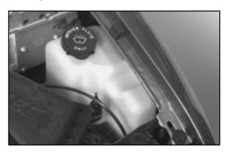
Open the cap labeled WASHER FLUID ONLY with the washer symbol on it. Add washer fluid until the tank is full.
