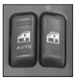
Press the side of the switch with the down arrow to lower the window.
