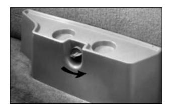
This is the jack cover for the extended cab. The cover for the regular cab is similar. To remove it, turn the plastic wing nut counterclockwise. Remove the jack cover.
