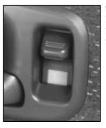
To unlock the door, slide the lever on your inside door up. You will see a red area on the lever.
