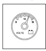
When your engine is not running, but the ignition is on (in RUN), this gage shows your battery's state of charge in DC volts.
