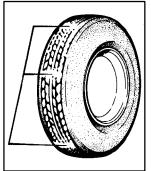
One way to tell when it's time for new tires is to check the treadwear indicators, which will appear when your tires have only 1/16 inch (1.6 mm) or less of tread remaining.
