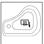
Your vehicle may be equipped with heated outside rearview mirrors. When you operate the heated mirror button on your climate control system, the defogger will warm the mirrors to help clear them of ice, snow or condensation.
