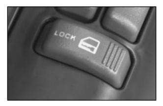
If your vehicle has power door locks, the switch is located on the armrest. Remove the ignition key and press LOCK to lock all the doors at once.
