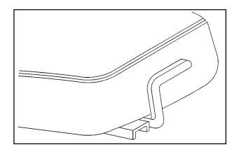
Move the lever under the front of the manual seat up to unlock it. Slide the seat to where you want it. Then release the lever and try to move the seat with your body to make sure the seat is locked into place.
