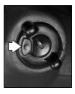
The key cannot be removed from the ignition of manual transmission vehicles unless the key release button is used.
