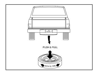
4. Make sure the tire is stored securely. Push, pull, and then try to rotate or turn the tire. If the tire moves, use the wheel wrench to tighten the cable.
