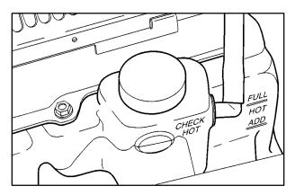
The vehicle must be on a level surface. When your engine is cold, the coolant level should be at ADD, or a little higher. When your engine is warm, the level should be up to FULL HOT, or a little higher.
