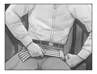
To make it shorter, pull the belt as shown until it is snug. Buckle and position it the same way as the lap part of the driver's safety belt (see "Driver Position" in the Index). Make sure the release button on the buckle is positioned so you would be able to unbuckle the safety belt quickly if you ever had to. To unlatch the belt, just push the button on the buckle.
