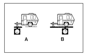
If you're using a weight-carrying hitch, the trailer tongue (A) should weigh 10 percent of the total loaded trailer weight (B). If you're using a weight-distributing hitch, the trailer tongue (A) should weigh 12 percent of the total loaded trailer weight (B).
