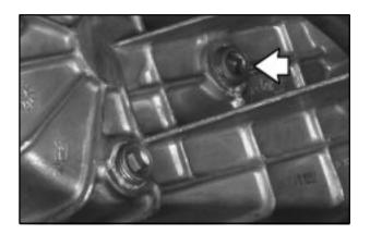
If the level is below the bottom of the filler plug hole, you'll need to add some lubricant. Add enough lubricant to raise the level to the bottom of the filler plug hole. Use care not to overtighten plug.
