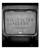
The access door for the remote oil filter is in the steering linkage shield assembly located under the radiator support. Twist the screw to unlock or lock the door. Make sure if you open the door, it is securely closed when you are finished.
