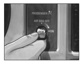
To turn the right front passenger's air bag on again, insert your ignition key into the switch, push in, and move the switch to the ON position.
