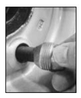
8. Put the nuts on by hand. Make sure the cone-shaped end is toward the wheel.
