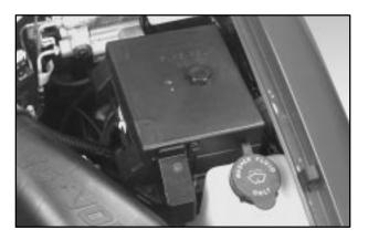
The fuse block is under the hood on the driver's side of the engine compartment.
