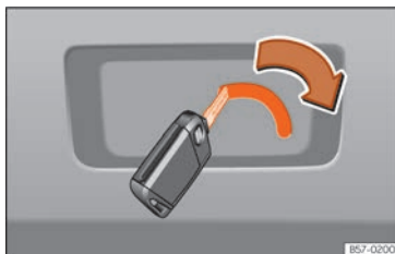
Fig. 11 Luggage compartment: manual release.
