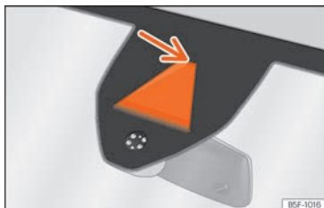
Fig. 266 On the windscreen: field of vision of the Lane Assist system camera.
