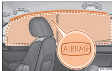
Fig. 34 Location of head-protection airbags.
