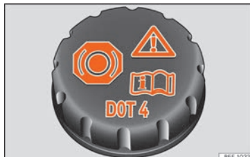
Fig. 65 Engine compartment: brake fluid reservoir cap.
