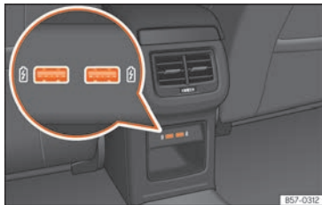
Fig. 237 Centre console, rear section: USB connectors.
