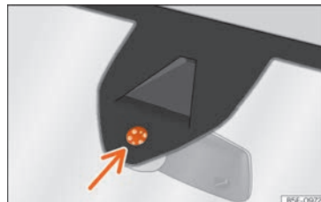
Fig. 157 Rain sensor sensitive surface
