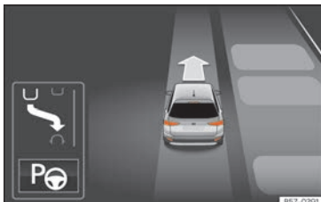
Fig. 282 On the instrument panel display: display of the assisted parking system with decreased visibility.
