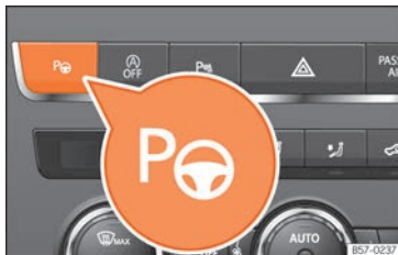
Fig. 280 In the centre console, top section: button to switch on the Park Assist system.
