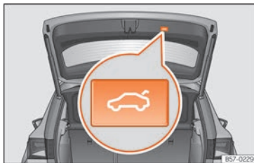
Fig. 145 Rear lid open: button to close rear lid immediately.
