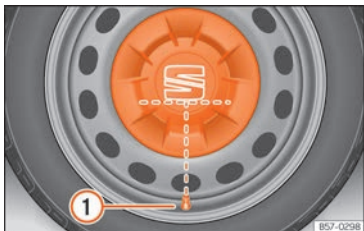
Fig. 74 Correct positioning of the central wheel trim for steel rims.
