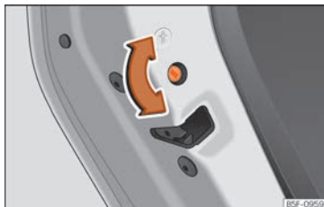
Fig. 143 Childproof lock on the left hand side door.
