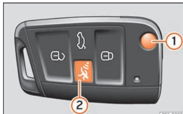
Fig. 137 Vehicle key with alarm button.
