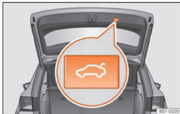
Fig. 9 Rear lid: button to close rear lid.
