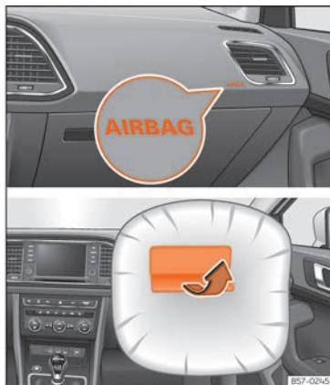
Fig. 27 Front passenger airbag located in dash panel.
