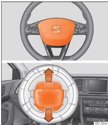
Fig. 26 Driver airbag located in steering wheel.
