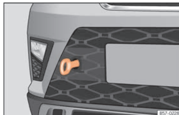
Fig. 102 Right side of the front bumper: towline anchorage screwed in.
