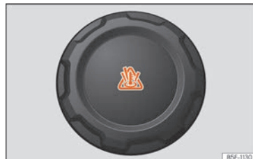
Fig. 64 Engine compartment: coolant expansion tank cap. »
