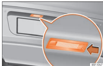
Fig. 118 In the rear bumper: number plate light.
