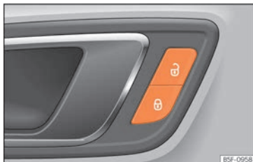
Fig. 5 Driver door: central locking switch.
