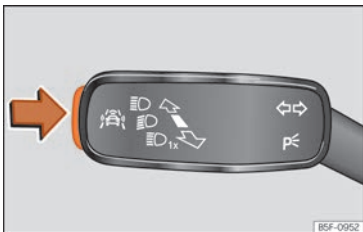
Fig. 134 On the turn light and main beam lever: key for driver assistance systems.
