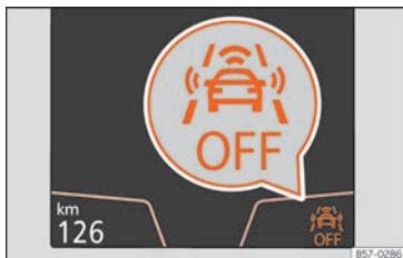
Fig. 256 On the screen of the instrument panel Front Assist switched off message.
