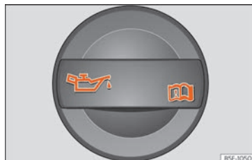
Fig. 63 In the engine compartment: Engine oil filler cap.
