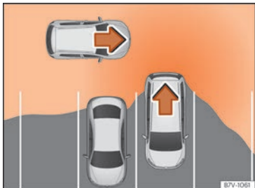
Fig. 275 Diagram of the parking assistant: detected area around the vehicle that is driving off.
