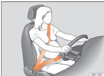
Fig. 97 Position of seat belt during pregnancy.
