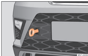
Fig. 80 Right side of the front bumper: towline anchorage screwed in.
