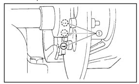
Brake pad wear indicator groove
