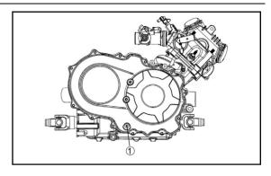
1. CVT Gear Box inspection hole
