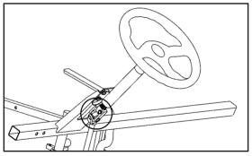
Lower universal joint, steering transmission shaft
