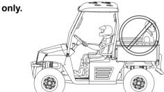
The total weight of operator, passenger, accessories, cargo, trailer tongue weight, and the vehicle itself must not exceed 2180lbs (989Kg).
