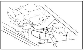
Engine oil drain bolt
