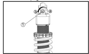
1. Compression damping force adjusting screw
