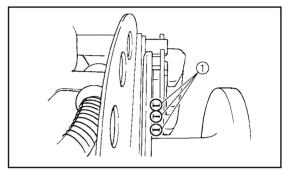
1. Brake pad wear indicator groove
