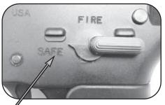
Safety lever in "SAFE" position. NOTE: You cannot put the firearm on "SAFE" unless the hammer is cocked!
