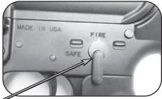
Safety lever in "FIRE" position. Pulling the trigger when the safety lever is in the "FIRE" position will result in the rifle firing if there is a round in the chamber! Exercise extreme caution when handling rifle in this condition.
