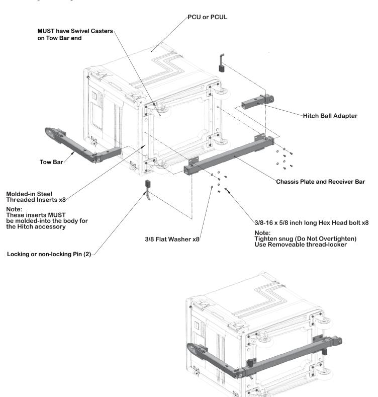
WARNING! Components and Cart, with installed Hitch are **NOT** intended for use on the STREET or HIGHWAY. Pulling speed should **NOT** exceed ten (10) miles per hour. When the Tow Bar is not in service, it should be pinned in the vertical position or completely removed from the cart to reduce a trip hazard.
