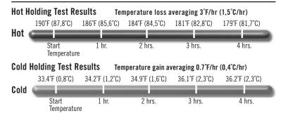
\*\*Based on test with 10 each 4" (10 cm) deep H-Pans<sup>™</sup> with GripLids<sup>®</sup> filled with hot water at starting temperature of 190°F (87,8°C) held in compartment with door shut. Water temperature dropped an average of only 3°F (-16,1°C) /hr.
