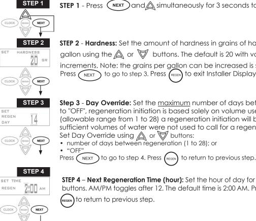
STEP 2 - Hardness: Set the amount of hardness in grains of hardness as calcium carbonate per gallon using the 🛕 or 🕅 buttons. The default is 20 with value ranges from 1 to 150 in 1 grain increments. Note: the grains per gallon can be increased is soluble iron needs to be reduced. Press (NEXT) to go to step 3. Press (REGEN) to exit Installer Display Settings.
