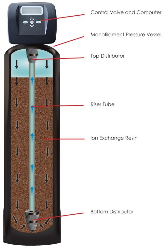
The system must be BYPASSED, DEPRES-SURIZED, and DE-ENERGIZED before assembling or performing mechanical repairs
