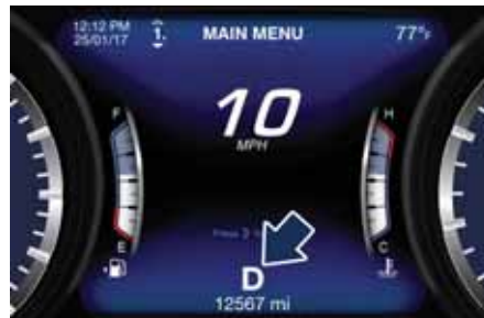
Transmission status is visible on the lever and on the lower part of the Instrument cluster display.
