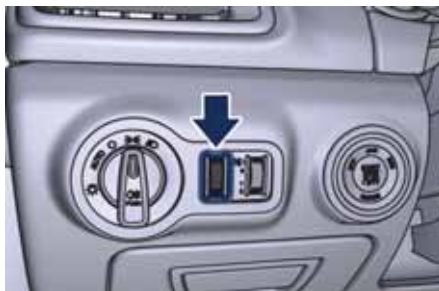
The regulation device rotates from position "0" upward and back
