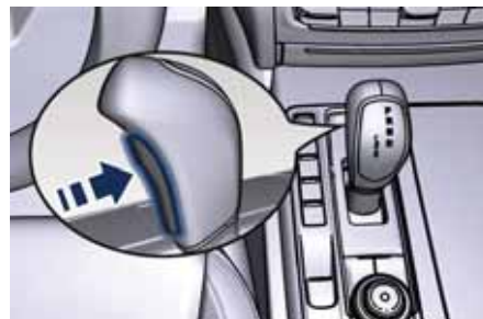
Transmission status is visible on the lever and on the lower part of the Instrument cluster display.
