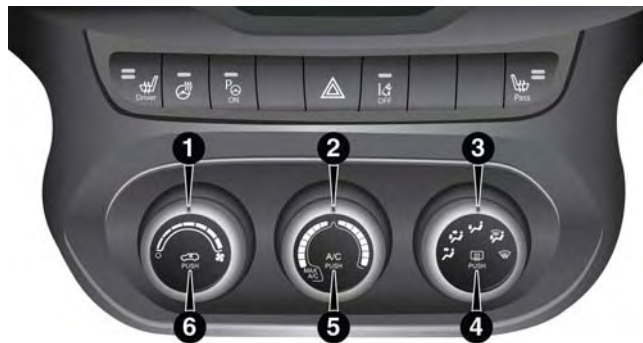
Manual Temperature Controls (MTC)
