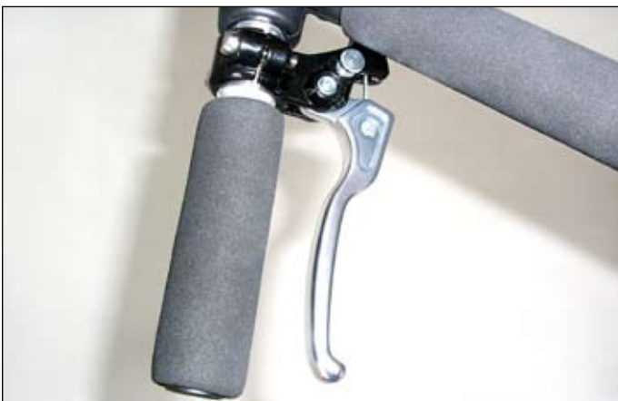
Brake lever in the parked position
