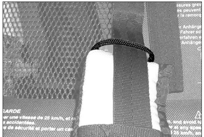
L: Sleeve through both webbing loops and the top cord loop.
