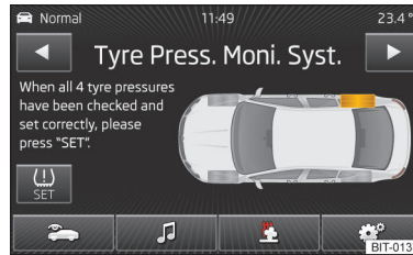
Fig. 46 Tire pressure monitor - Display example: Check the right rear tire and its filling pressure
