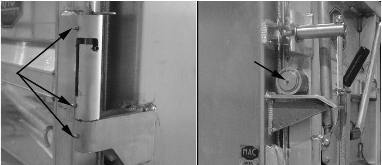
Figure 8-4 Side Swing Rear Gate Hinges And Roller Grease Fittings
