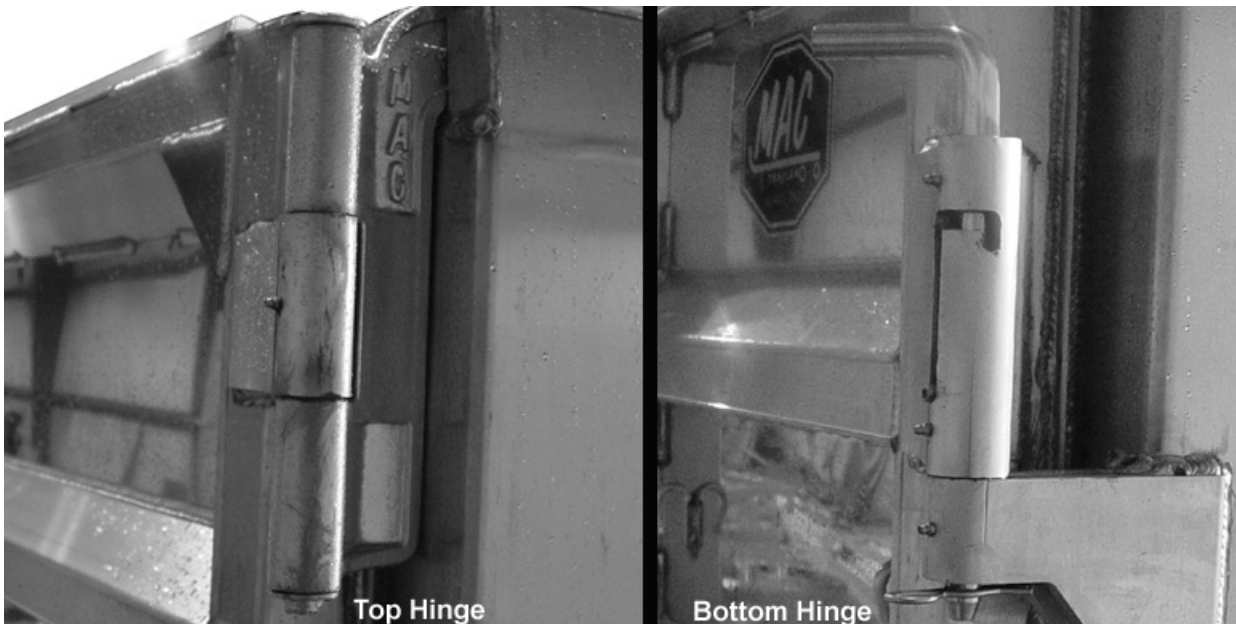
Figure 5-3 Side Swing Hinges Properly Engaged
