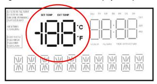
This area indicates the internal (or external) temperature and can be programmed to display in either "Celsius" or "Fahrenheit".
