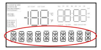
This line is used to show extra information in the basic mode; error messages to provide interface when going through menus in advanced mode. Longer text lines are scrolled to the left on the display.
