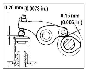
Valve clearance adjustment values are the same for both the intake and the exhaust.
