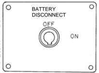
the "on" position. Twelve volt DC power now moves from battery, through converter to coach. When you wish to charge the battery by power converter, the switch must be in "on" position providing you have 120 volt AC power available.
