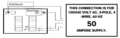
service yet serve two separate banks as the external sticker indicates. A 50 amp main breaker will distribute current to separate banks, verifying 240 volts are present. There are no 240 volt appliances in this coach.
