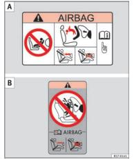
Fig. 28 Airbag stickers - version 1: on the passenger-side sun blind (A) and on the rear frame of the front passenger's door (B).
