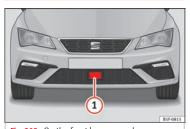
Fig. 203 On the front bumper: radar sensor.
