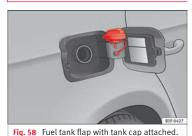
The flap that covers the tank cap is unlocked and locked automatically using the central locking.
