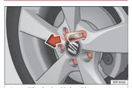
Fig. 70 Wheel: wheel bolts with caps.
