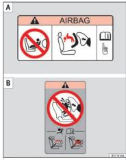
Fig. 29 Airbag stickers - version 2: on the passenger-side sun blind (A) and on the rear frame of the front passenger's door (B).
