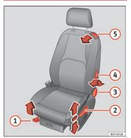
Fig. 13 Front seats: manual seat adjustment.
