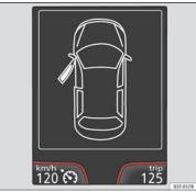
Fig. 50 On the instrument panel display: door open.
