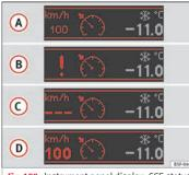
Fig. 199 Instrument panel display: CCS status indications.
