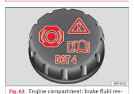
ervoir cap. The brake fluid reservoir is located in the en-
