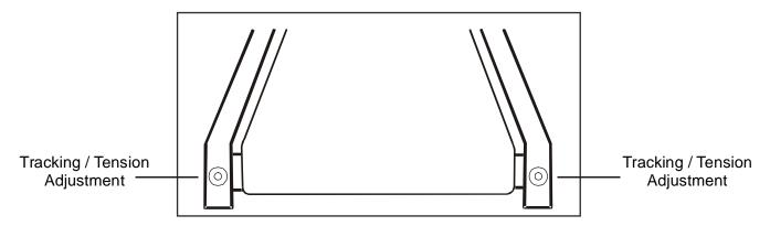
**Note:** Adjustment is through small hole in end cap.
