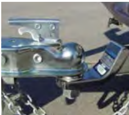
Fig. 2: Coupler on ball with latch in proper lock position.
