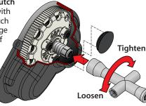
noise. Remove the rubber slipper clutch plug on the transmission cover in order to adjust the slipper. Use the 4-way wrench to turn the adjusting nut clockwise to tighten and counter-clockwise to loosen. Place the model on a high-traction surface, such as carpet. Adjust the slipper so that you can hear it slip for approximately two feet from a standing, full throttle start.
