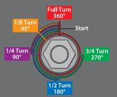
Do not run your model with the slipper clutch adjusting spring fully compressed. The minimum recommended slipper clutch setting is 1/2 turn counter-clockwise from fully compressed. Gearing Compatibility Chart: The chart below shows a full range of gear combinations. This does NOT imply that these gear combinations should be used. Over-gearing (bigger pinions, smaller spurs) can overheat and damage the motor and/or speed control. Items in black will fit 540 motors only (not Titan 12T).
