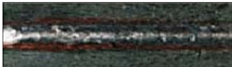
VOLTAGE TOO HIGH
