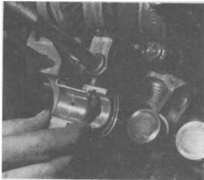
24.8 Fit the 3 crankshaft bearing shells. The rear one is flanged.
