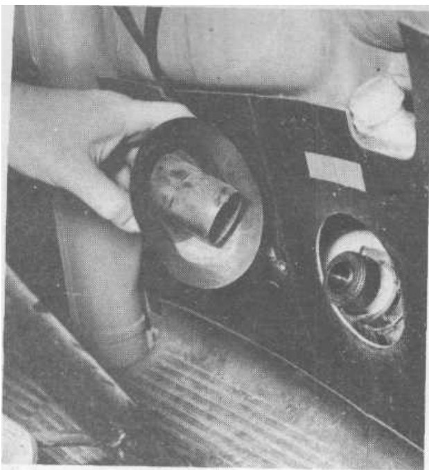
The windscreen washer reservoir is mounted on the vertical panel in the front of the cab just below the brake fluid reservoir.
