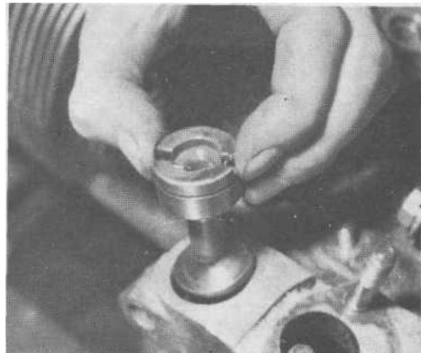
6.8a Replacing the distributor drive shaft. Note the fuel pump drive cam on the shaft
