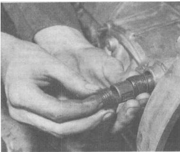
4.8d Make sure the bush and seal do not come out on the inside like this
