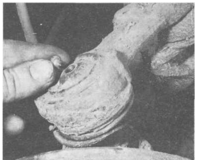
4.1 The plug may be replaced by a grease nipple
