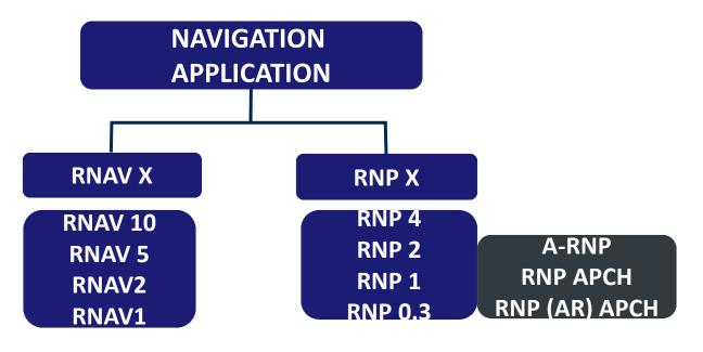
X = Navigation Accuracy in NM 95% of flight time
