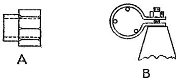
Fig. 1—Special threaded nut (A) and keyed clamp (B) for mechanism for remotely adjusting antenna-element lengths.
