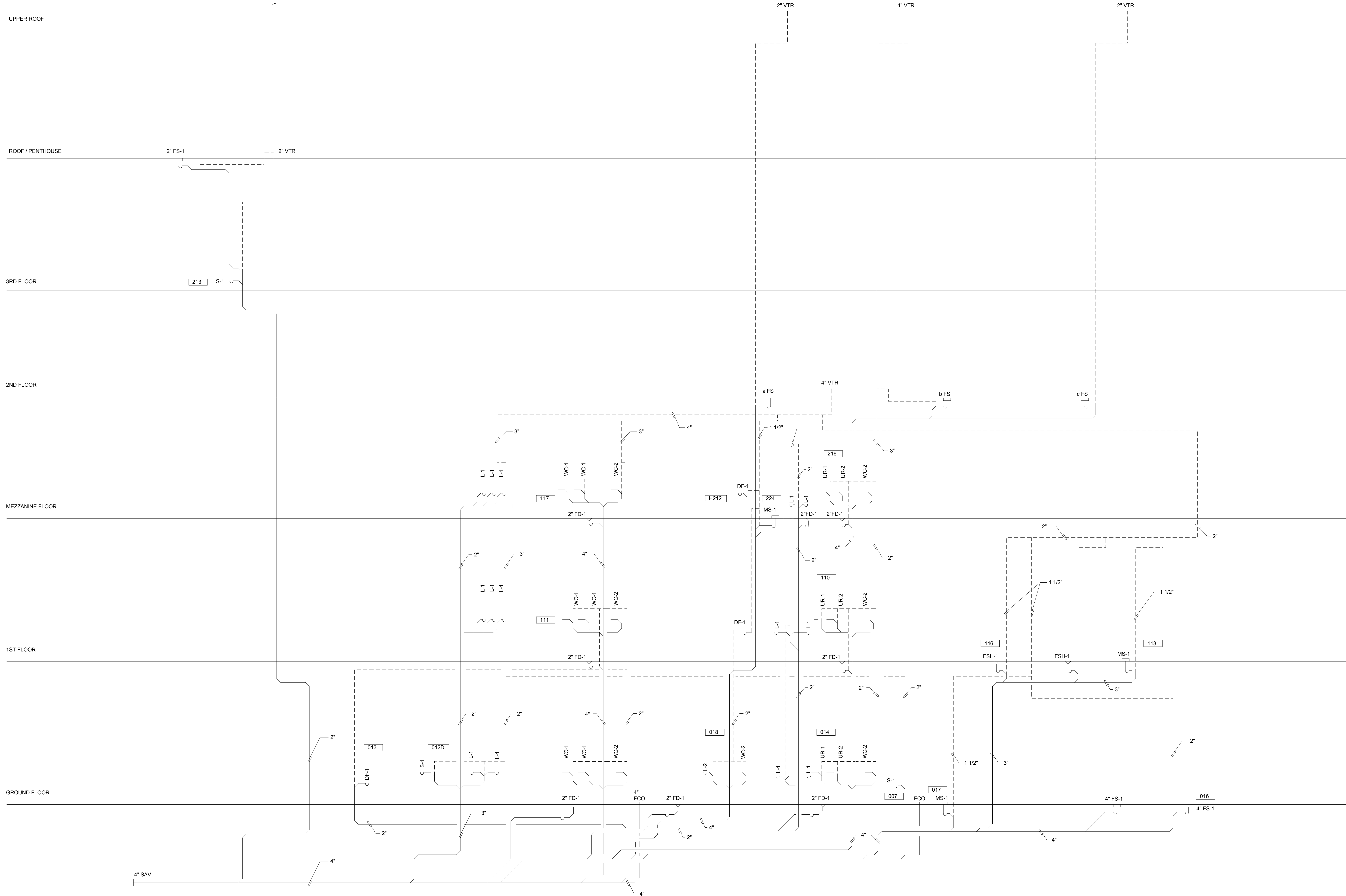
1 WASTE AND VENT RISER DIAGRAM SCALE: 1/8" = 1'-0"
