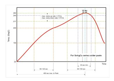
Fig 2. Infrared soldering profile
