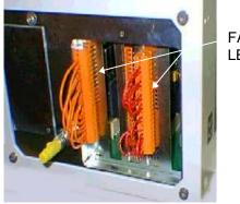
FAULT LEDs AO8 Board provides 3-LED troubleshooting status lights. The status lights provide information on what functions occur when a status light is illuminated. Status lights illuminate orange, red or green.
