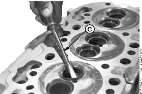
Valve Seat Insert Removal
