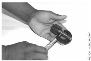
Measuring Drive Shaft OD for Wear
