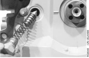
NOTE: Mark and identify location of timing gear cover hardware before removal to aid in reassembly.
