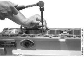
Marking Cylinder Liner Location/Position
