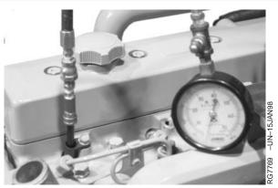
Compression Tester in Nozzle Bore
