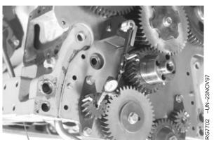
Measuring Balancer Shaft End Play-4-Cylinder
