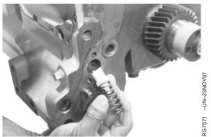
Oil Bypass Valve and Spring
