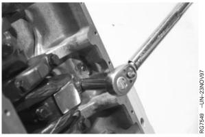
Connecting Rod Bearing Cap Screws
