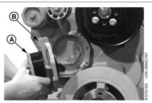
Water Pump with Pulley on Timing Gear Cover
