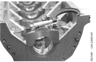
Measuring Cylinder Block Main Bearing Bore
