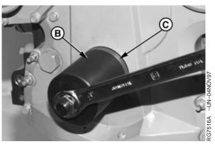
Front Crankshaft Oil Seal Tool
