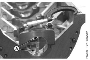
Measuring Main Bearing Cap ID Assembly
