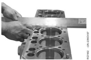
Measuring Cylinder Block Top Deck Flatness
