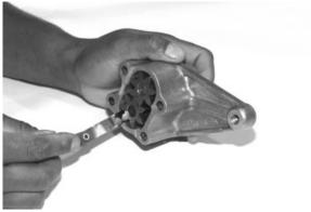
Checking Gear-to-Pump Housing Radial Clearance
