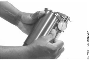
Measuring Liner Flange Thickness
