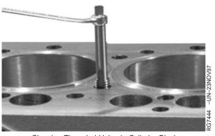
Cleaning Threaded Holes in Cylinder Block
