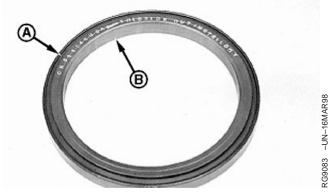
Crankshaft Rear Oil Seal and Wear Sleeve
