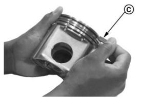
Piston Ring Groove Wear Gauge
