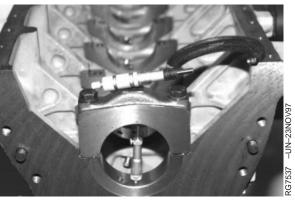
Measuring Assembled Main Bearing Cap ID
