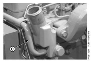
Thermostat Cover-to-Water Pump Tube
