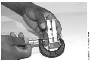
Measuring Main Thrust Bearing Width
