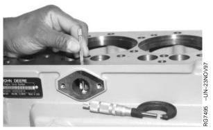
Fuel Supply Pump Push Rod Bore
