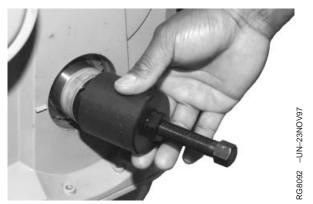
Crankshaft Wear Sleeve Removal Tool
