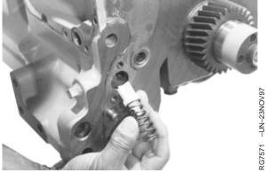
Oil Bypass Valve and Spring
