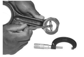
Measuring Connect Rod Pin Bore ID
