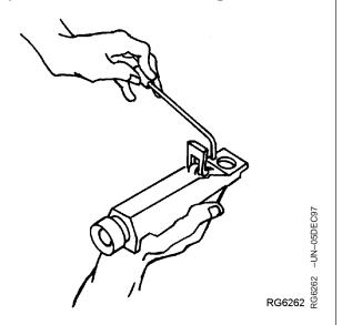
Maintaining the correct coolant conditioner concentration (SCAs) and freeze point is essential in your cooling system to protect against rust, liner pitting and corrosion, and freeze-ups due to incorrect coolant dilution.
