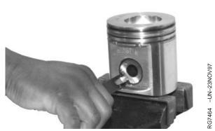
Piston Pin Snap Ring Removal
