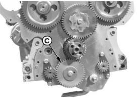
Lower Idler Gear and Thrust Washer
