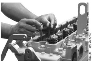
Rocker Arm Assembly Installation
