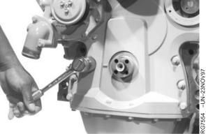
Oil Pressure Regulating Valve in Timing Gear Cover
