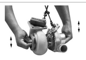
Radial Bearing Clearance Test
