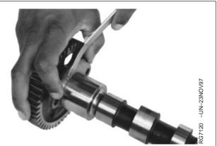
Measuring Camshaft Thrust Plate
