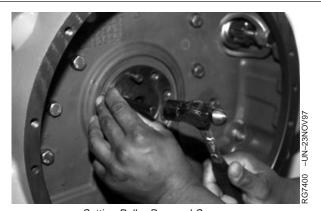
Setting Puller Removal Screws
