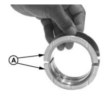
Assembled Main Thrust Bearing
