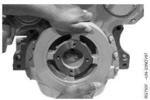
Vibration Damper—6-Cylinder Engine
