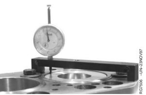
Piston Protrusion above Block Deck
