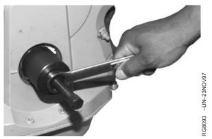
Crankshaft Wear Sleeve Removal Tool
