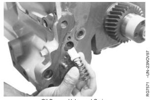
Oil Bypass Valve and Spring
