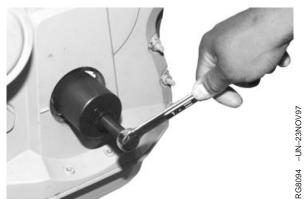
Crankshaft Wear Sleeve Removal Tool
