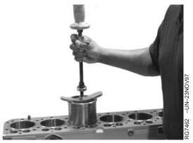
Pulling Cylinder Liners Out of Block
