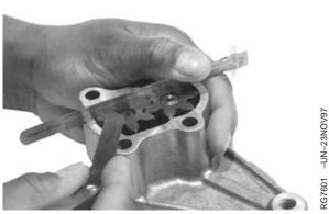
Checking Gear-to-Pump Cover Axial Clearance
