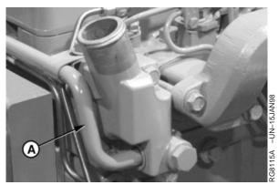
Thermostat Cover-to-Water Pump Tube
