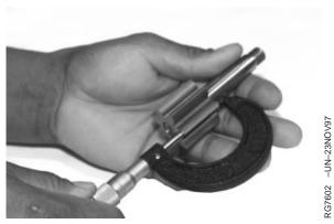
Checking Gear Thickness
