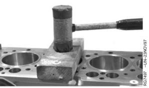
Install Cylinder Liner in Block
