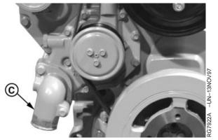
Water Pump Inlet Elbow
