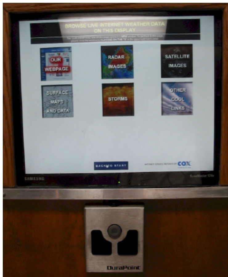
FIG. 4. The web browser display. The photograph shows the home page where the user selects from six options to begin their browsing experience. The mouse is manufactured by Interlink Electronics Corp. ( http://www.interlinksensors.com/ ) and is designed for a harsh, high-use environment.
