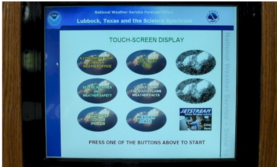
FIG. 3. The touch screen display. The screen is a 17" LCD monitor manufactured by Tyco Electronics Corporation ( http://www.elotouch.com/ ). This model came with USB drivers for operability with a PC running Microsoft Windows.
