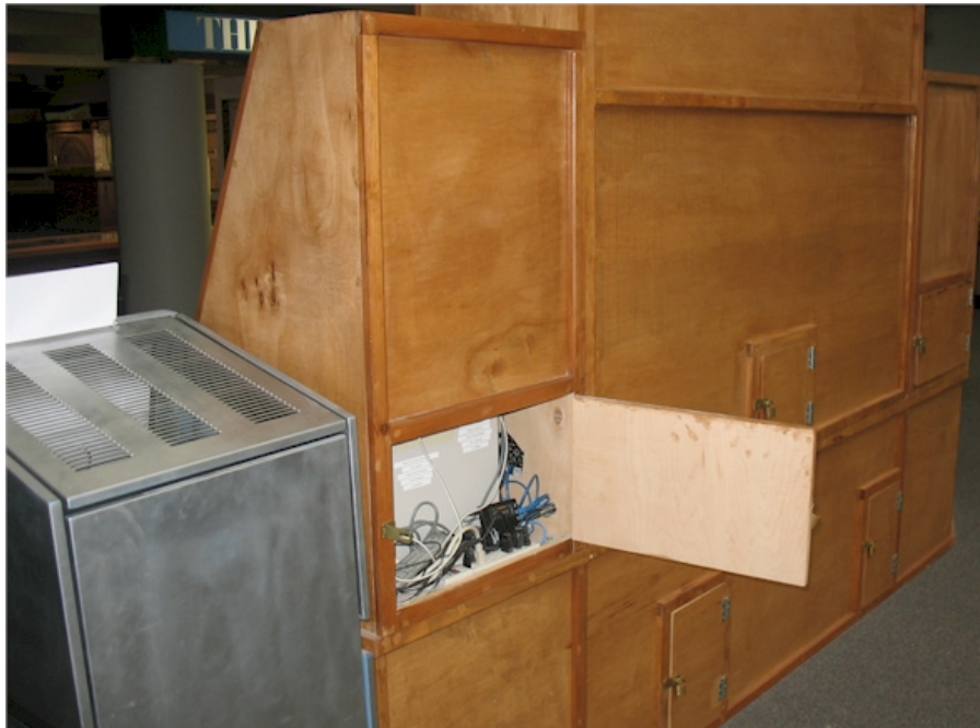
FIG. 7. The back of the display showing the various compartment access panels. The open panel shows the location of the web browser and the presentation PCs.
