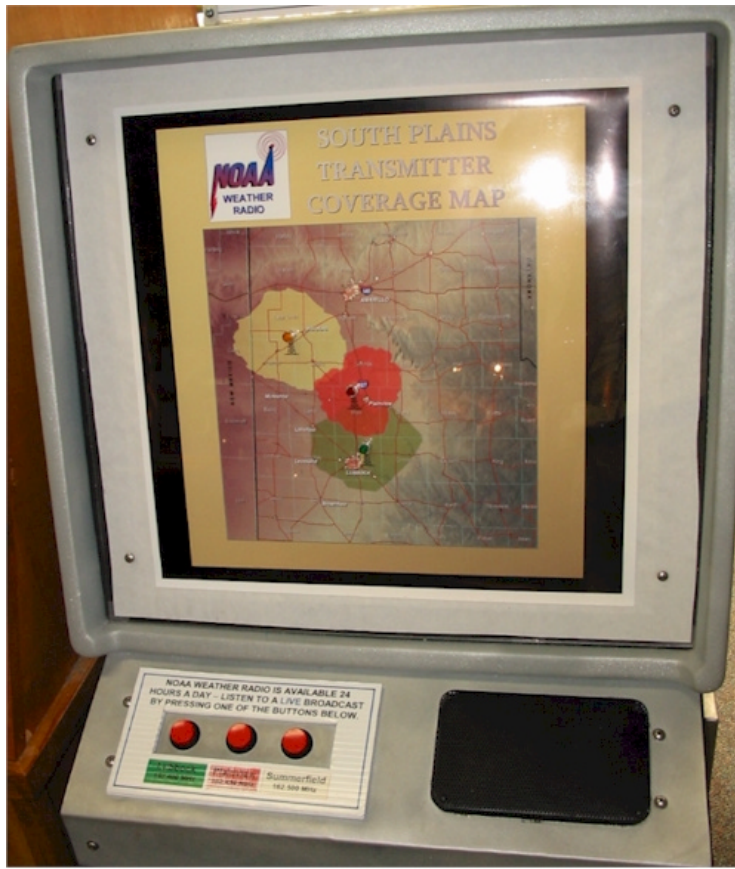
FIG. 6. The NOAA Weather Radio display. When a button is depressed, the program audio is played, and the appropriate transmitter lights up on the map.
