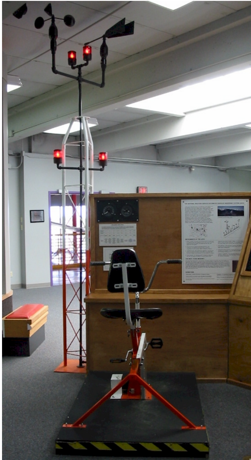
FIG. 5. The instrumented tower and bicycle display. The fan is barely visible in the upper-left corner. Another fan blows air out of the top of the main enclosure to gently rotate the wind vane.
