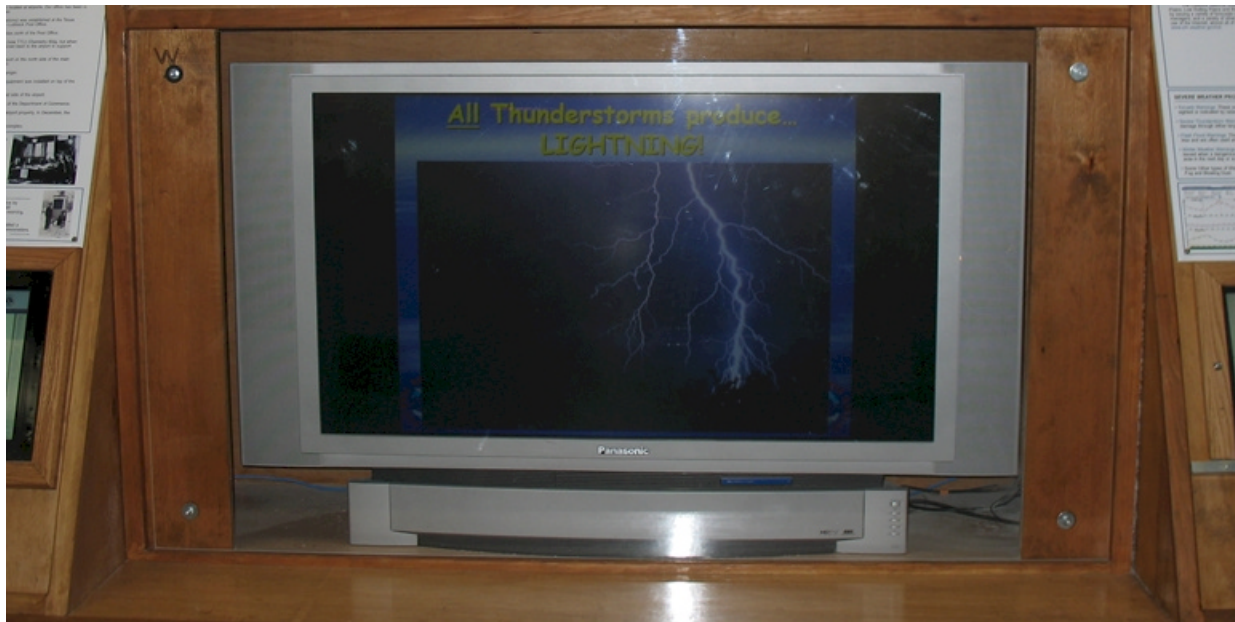
FIG. 2. Close-up of the LCD monitor. The screen is protected by a sheet of acrylic glass installed in front of the monitor. The presentation is produced and displayed using Microsoft PowerPoint in kiosk mode.
