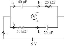
The reading of voltmeter at any instant =  $\Delta V_{40\mu F} - \Delta V_{50k\Omega} = 5 \left(1 - e^{-\frac{t}{\tau}}\right) - 5e^{-\frac{t}{\tau}}$
