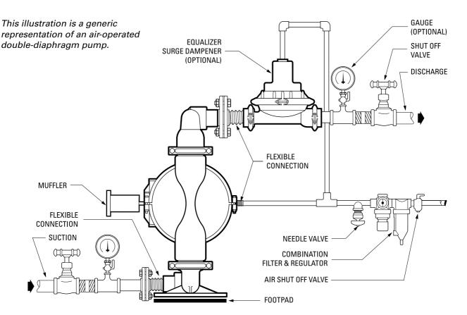
**NOTE**: In the event of a power failure, the shut off valve should be closed, if the restarting of the pump is not desirable once power is regained.
