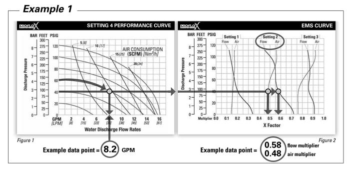
This is an example showing how to determine flow rate and air consumption for your Pro-Flo  $X^{\text{TM}}$  pump using the Efficiency Management System (EMS) curve and the performance curve. For this example we will be using 4.1 bar (60 psig) inlet air pressure and 2.8 bar (40 psig) discharge pressure and EMS setting 2.
