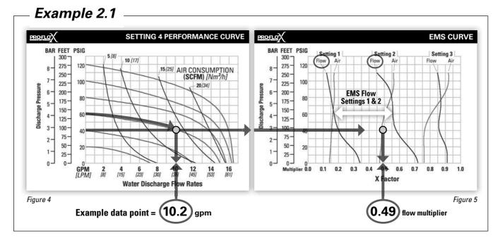
This is an example showing how to determine the inlet air pressure and the EMS setting for your Pro-Flo  $X^{\text{TM}}$  pump to optimize the pump for a specific application. For this example we will be using an application requirement of 18.9 lpm (5 gpm) flow rate against 2.8 bar (40 psig) discharge pressure. This example will illustrate how to calculate the air consumption that could be expected at this operational point.
