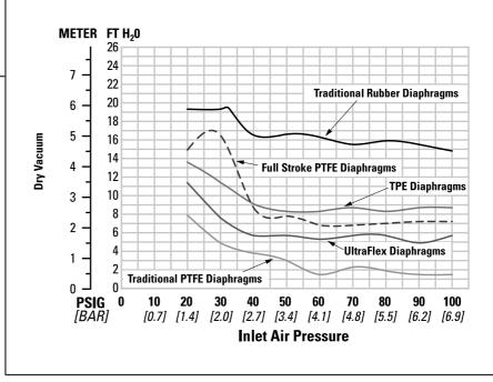
Suction lift curves are calibrated for pumps operating at 305 m (1,000') above sea level. This chart is meant to be a guide only. There are many variables which can affect your pump's operating characteristics. The
