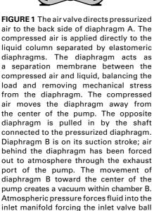
off its seat. Liquid is free to move past the inlet valve ball and fill the liquid chamber
