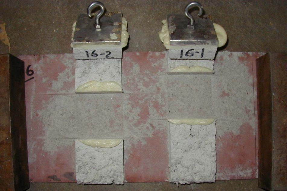
Test 1- Adhesive failure
