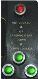
The landing gear indicators will show 3-green when all three gears are down and locked. Otherwise the will show red (in transit, but not locked) or they will be dark (gear up). If the gear handle is in the down position, and all three gears are not locked, the Gear Not Locked warning indicator will illuminate red.
