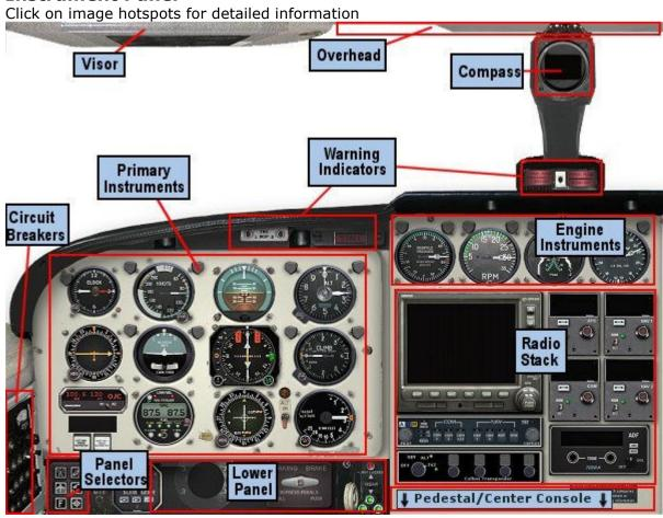
The instrument panel is designed to be functional and professional and will accommodate complete instruments and avionics. The owner's individual needs can surely be fulfilled with the wide selection of optional equipment available.
