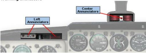
Left Annunciators Center Annunciators: Engine Out Low Fuel Flow Indicators Low Oil Pressure
