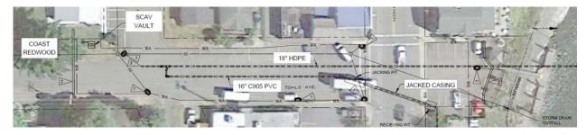
Photo: Pump Station Connection Piping in Nehalem
