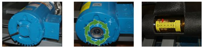
To confirm flow ,check the Flow Meter. If no flow is indicated, it is likely there is an air lock in the pump and you will need to bleed the air from system. Confirm both valves are open and try cycling the power to the pump OFF and ON . If still no flow, turn power off and carefully open the plug located on the stainless steel head of the pump, bleed air from pump head and re-tighten pump head plug.
