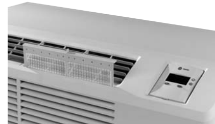
Figure 19. Intake air filter removal is through top of unit. Inspect and clean filters monthly for proper unit operation.
