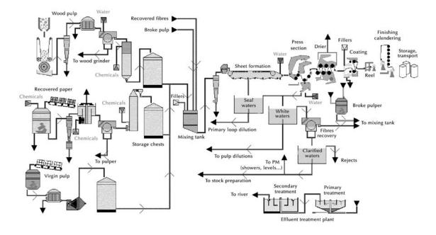
A board machine often has several formation devices in the wet end (headboxes and wires) producing a multi-ply sheet, combined on the forming table and press. Basis weight of the boards can be as high as 500 g/sq.m, whereas the printing and writing papers are usually 40-120 g/sq.m. Paper and board machines are each different – the size of the production capacity and technology varies. Each one is tailored to the specification of the paper mill.
