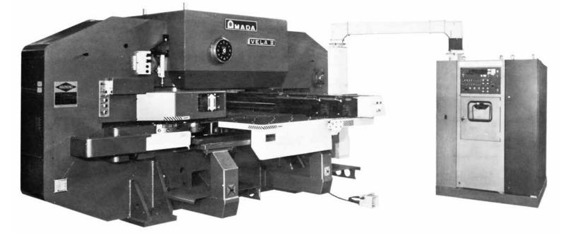
This 30 ton Vela II Amada Machine shapes and perforates our side panels with computer directed programming accurate to + .001".
