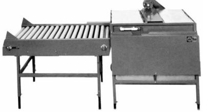
OVER-ALL LENGTH = 9' ONE  $\frac{1}{2}$  HP MOTOR AND ONE  $\frac{1}{4}$  HP GEARMOTOR RUN MACHINE
