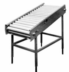
Drip pan Add \$125 The Roller Conveyor provides an excellent space for inspecting and sorting produce. Each piece of fruit or vegetable turns as it moves along so workers can see every side of it. Comes complete with gearmotor. Two people can work each side if necessary, but normally only one is needed.
