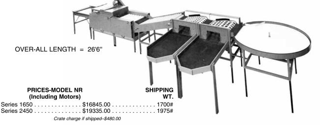
An example of how our well engineered units fit together to produce a complete tomato packing machine. Notice use of our waxer, sizing units fitted with rubber sizing belts and side delivery conveyors.
