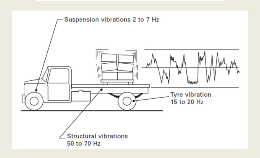
Stack resonance on a vehicle.
