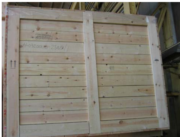
Photo shows: End of the box with additional stiffening elements
