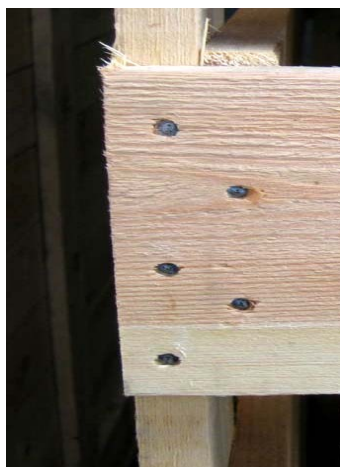
Photo shows: Method used for nailing corner joints when assembling the crate. Through the side board, there is a row of 3 nails for tacking the vertical end board and a row of 2 nails for tacking at the end of the horizontal end board.
